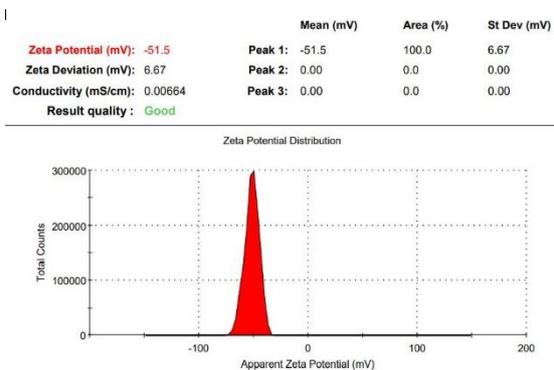
**Fig 4:** Zeta potential of the Nano-lignin Urea (Zeta potential -52 mV)
